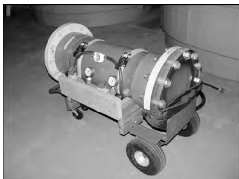
Figure 3. Hyperbaric chamber and secondary manifold (not in view) attached to a hand truck for ease of operation and portability.
