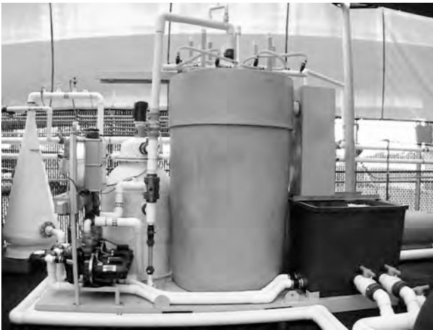
Figure 2. Example of a recirculating water treatment system.
