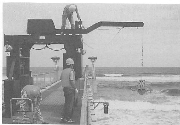
Figure 3. Sampling of bottom sediment using the Smith-McIntyre grab hoisted by a crane.
