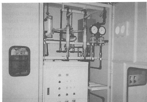
Figure 9. Interior arrangement of the precision filter unit showing a pair of hollow yarn film tubes (upper middle) with the pressure gauges (upper right).
