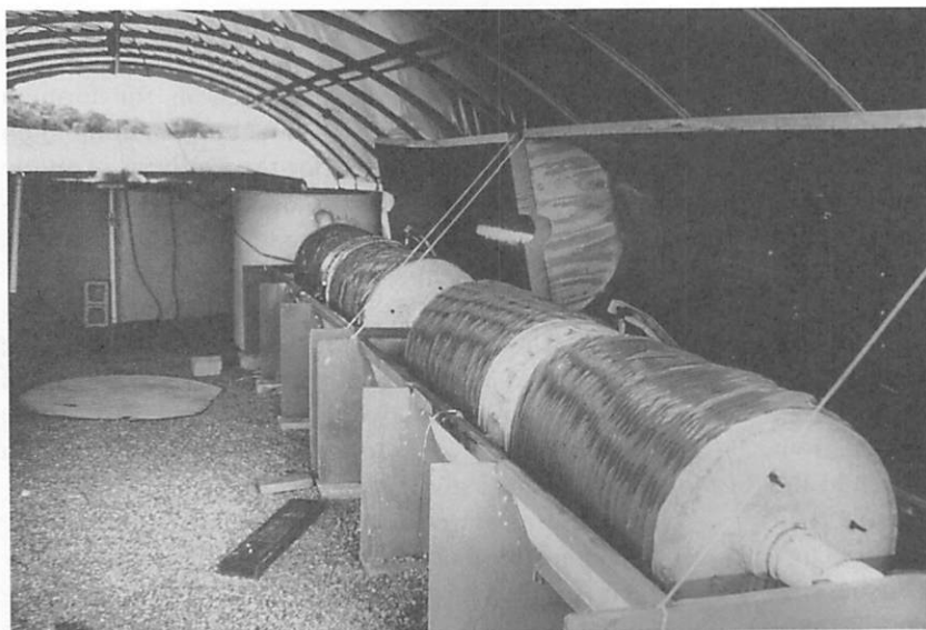
Figure 3. Rearing Tank (Left), Clarifier, and Two Rotating Biological Contactors of a Commercial-Scale Integrated System.
