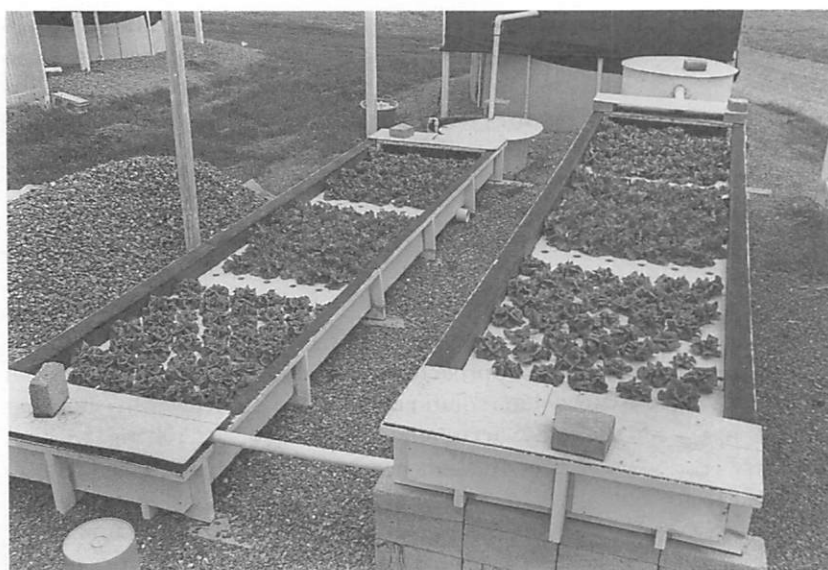
Figure 2. Experimental Integrated System Showing Rearing Tank (Background), Clarifier (Right), Hydroponic Tanks, and Reservoir (Left).
