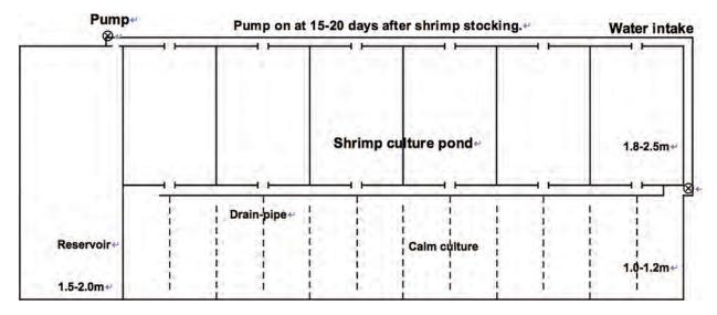
Fig. 6. Schematic diagram of the recirculating system for shrimp and clam culture in Zhejiang Province.
