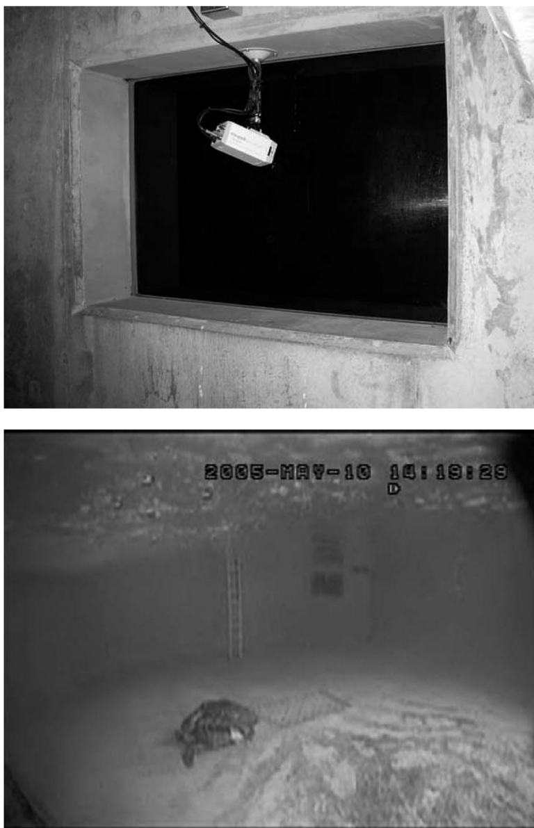
Fig. 3-1. Photographs of a highly sensitive camera fixed on the edge of the observation window (upper) and image of an observation of mating behavior in the 250kL tank (lower).
