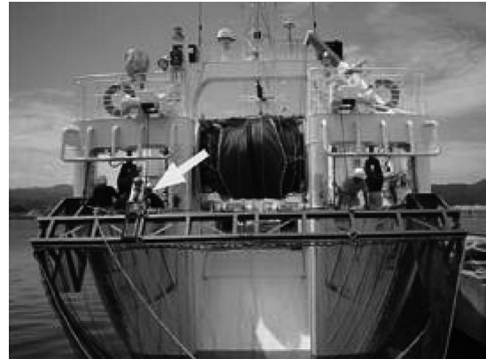
Fig. 1. Dredge net 'Beni-Zuwai Type 1' setting at stern of R.V. Tanshu-maru. The arrow indicates net-recorder.
