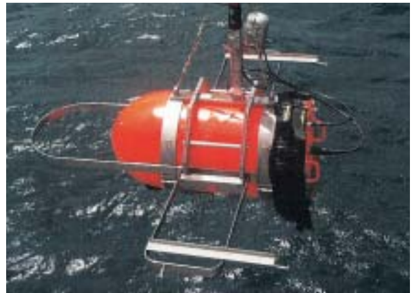
Fig. 63. Experimental setup of the test bench. The quantitative echo sounding system with split-beam transducer of 70kHz, and stereo video camera system are equipped in it. The black belt rounded test bench is weight for balance and the sensor unit for depth, temperature, roll and pitch angles is attached to the cable.
