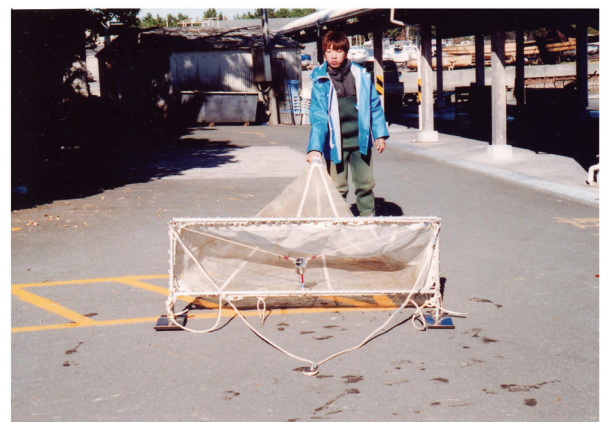
Fig. 3. Sledge net used for towing at bottom of coastal area
