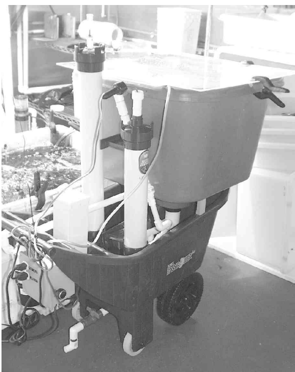
Fig. 6. Semi-square tank with recirculating pump, UV sterilizer and particulate filter as used for spray culture in controlled environment room
