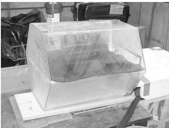
Fig. 4. Hexagonal chamber used for spray culture in greenhouse environment
