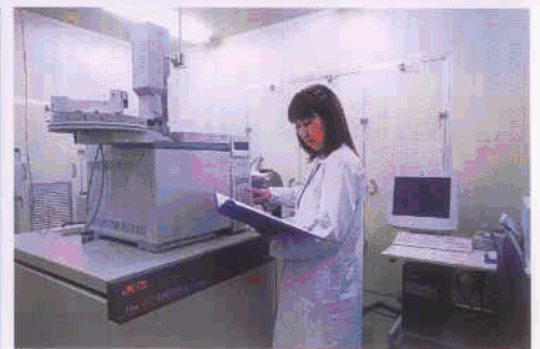
環境汚染物質の超微量分析。 Analysis of environmental pollutants by HRGC/HRMS.
