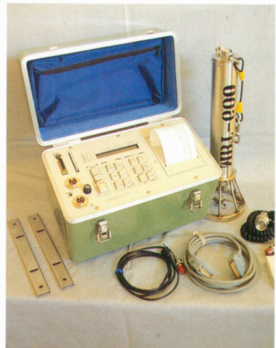
Electronic bathythermograph system for voluntary observation ships.
