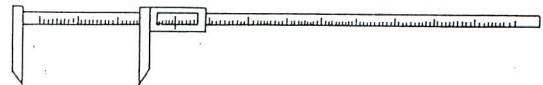
図3. 測定に用いたマルパス(上)と木製ノギス(下)。 Fig. 3. Outside calipers (upper) and wooden slide calipers (lower) for measuring the fishes.
