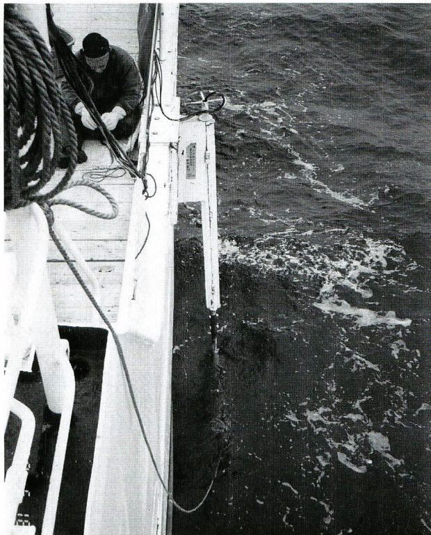
Appendix Figure 5. A pole with three hydrophones equipped on the starboard of the research vessel.
