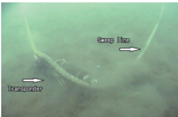
Fig. 9 The transponder buried with the seabed sand during drawing process
