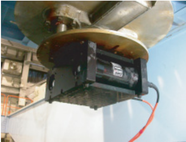
Fig. 3 Stereo camera frame for indoor tank experiment. The frame reproduces the same camera arrangement as J-QUEST pressure housing.
