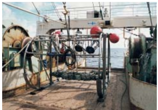
Fig. 2 Photograph of the deep-sea video monitoring system on a towed sledge on the R/V No.7-Kaiyo-maru.
